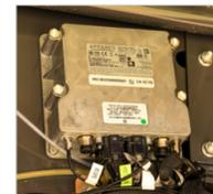
**ACM and Bale Link Status:** The AGCO Connectivity Module (ACM) is the telemetry device used to transmit data from baler to the cloud. The connection and subscription status of both are displayed for the master account holder to manage.
